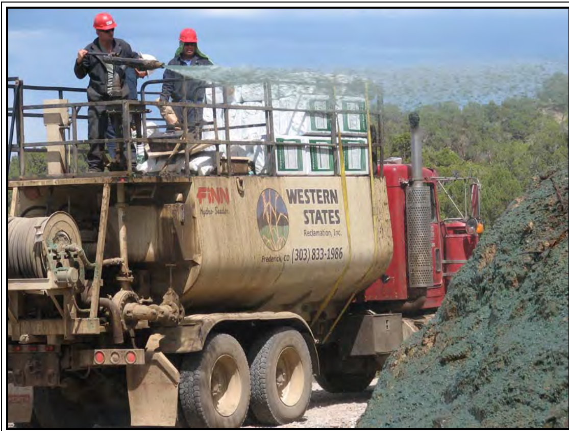
Photo 22: Hydroseeder – 3000 Gallon Tank
