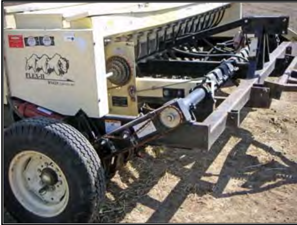
Photo 19: Seed Drill Gear Assembly
