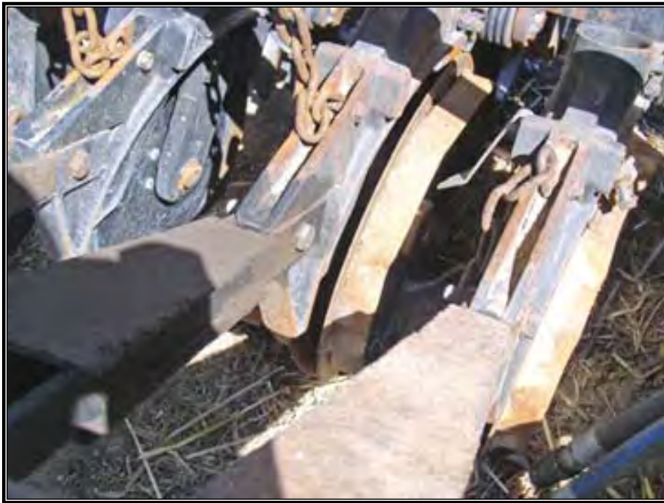
Photo 14: Close-up of Double Disk Furrow Openers and Depth Bands
